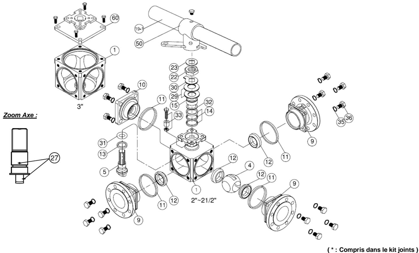
**ROBINET A TOURNANT SPHERIQUE 3 VOIES EN L INOX A BRIDES PN16**
