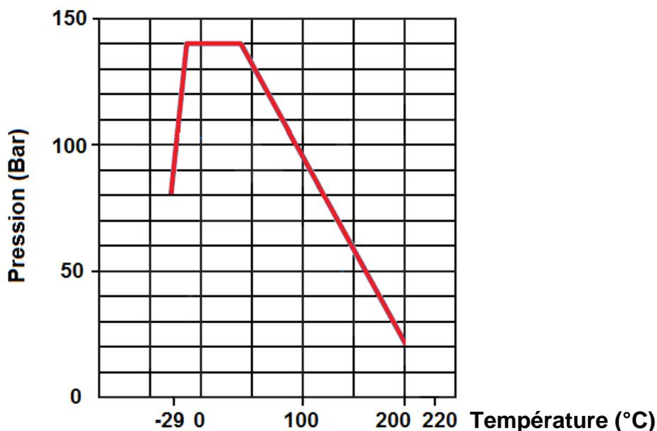
**ROBINET TOURNANT SPHERIQUE 3 PIECES ACIER A105N FORGE SWING 800LBS NPT-SW**
